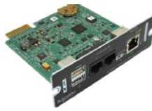
AP9641 UPS Network Management Card 3 with environmental monitoring (UPS with an embedded NMC have the same functionality as AP9641)
